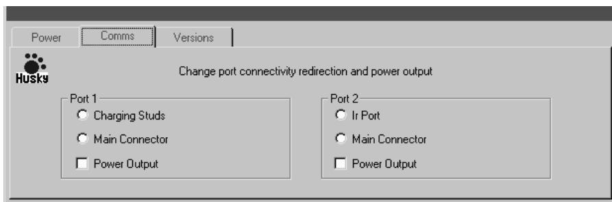
The Husky fex21 allows the COM1 port (Port 1) to be configured for use on the standard male 9-way D-type connector at the top left of the unit, or for use with the Vehicle Mount charging studs connector on the bottom left of the unit.
