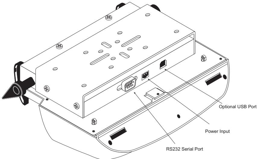
It is important to note that only certain pins of the serial port on the Vehicle Mount are connected – see the pinout diagram at the back of this booklet. This in no way impedes the ability of the serial port to transmit and receive data using ActiveSync, as long as the cable supplied with your fex21 is used.
