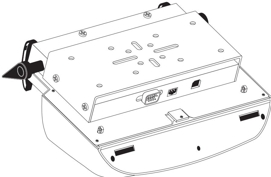
Two cable clamps and ties are provided on the back of the Vehicle Mount. These are to enable the power and communications cables to be fixed securely in position. We recommend that these ties are always used to prevent accidental damage to the cables.
