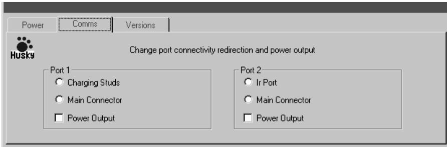
For use with the Desk Mount, COM1 should normally have the Charging Studs (located at the bottom left of the fex21 unit) selected. These studs connect through to the 9-way D-type connector on the rear of the Desk Mount and support the Desk Mount RS232 DTE communications port.
